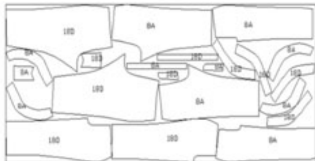
cal garment wastage and the simulated garment wastage. Pant A- marker 3a, Marker length -123.8. Layer length - 125.8 inches
